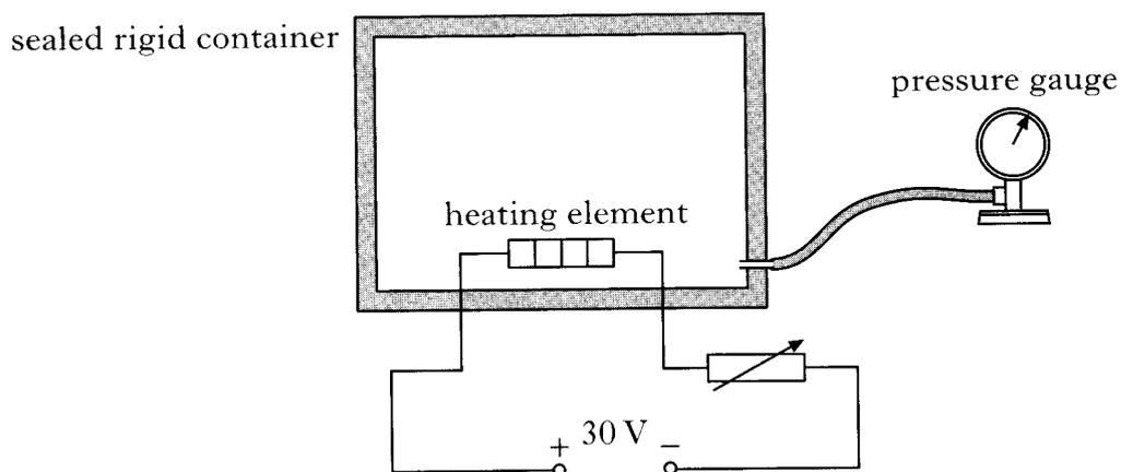
The heating element is used to raise the temperature of the gas.
