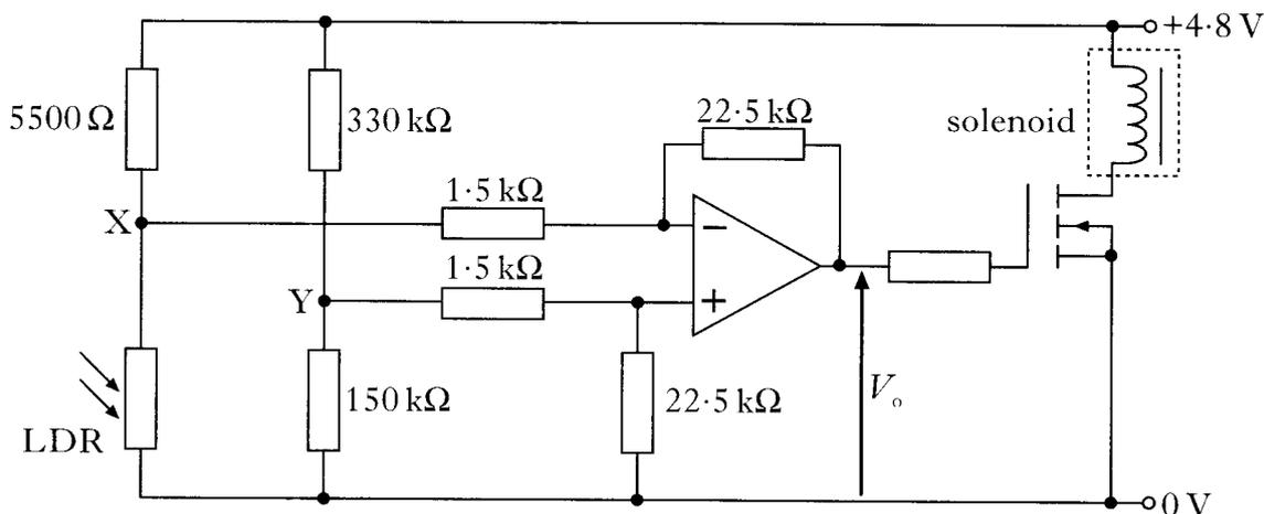
The potential at Y is  $1.50\ \text{V}$ . When the washing machine is filling with water, the narrow beam of light illuminates the LDR, the bridge is unbalanced and the potential at X is  $1.28\ \text{V}$ .
