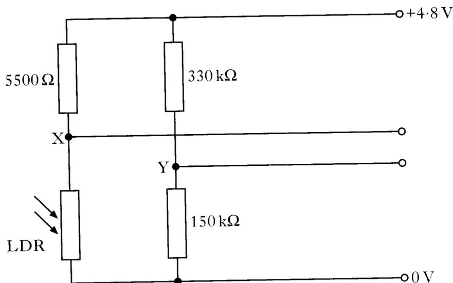
When the water in the machine is at the maximum level, the bridge is balanced.
