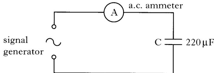
The signal generator is adjusted to give a peak output voltage of 12 V at a frequency of 300 Hz. The internal resistance of the signal generator and the resistance of the a.c. ammeter are negligible.
