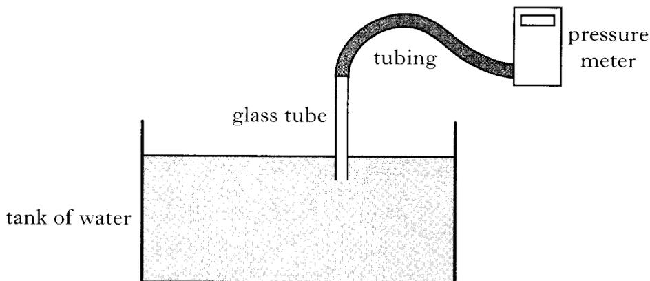
The pressure meter is set to zero before the glass tube is lowered into the water.
