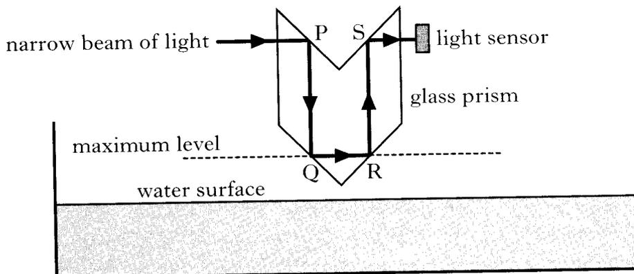
When the water in the machine is below the maximum level indicated in the diagram, the light sensor is illuminated by the narrow beam of light.
