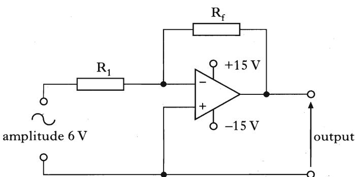
Which values for resistors  $R_1$  and  $R_f$  will produce an approximate square wave output?
