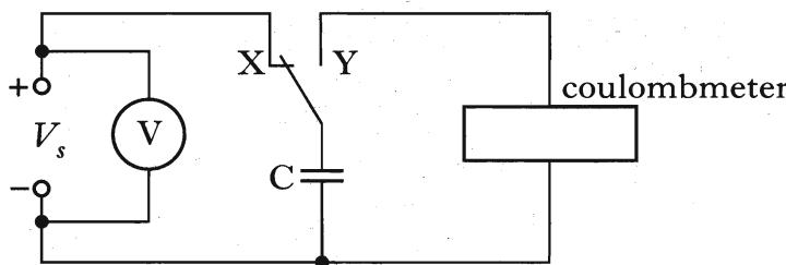
When the switch is in position X, the capacitor charges up to the supply voltage,  $V_s$ . When the switch is in position Y, the coulombmeter indicates the charge stored by the capacitor.
