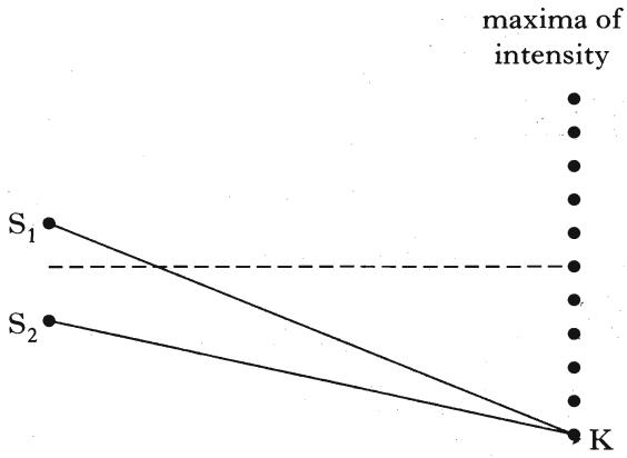
The path difference  $S_1K - S_2K$  is 154 mm. The wavelength of the waves is
