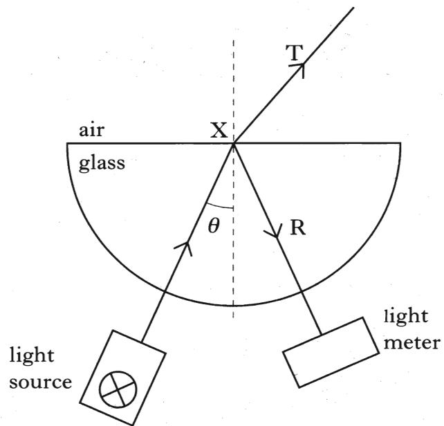
The student uses a light meter to measure the intensity of ray R as angle  $\theta$  is changed.
