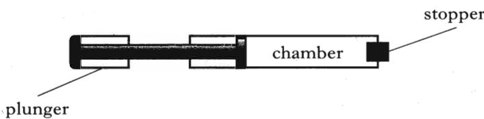
The plunger is now pushed in slowly causing the air in the chamber to be compressed. As a result of this the pressure of the trapped air increases.
