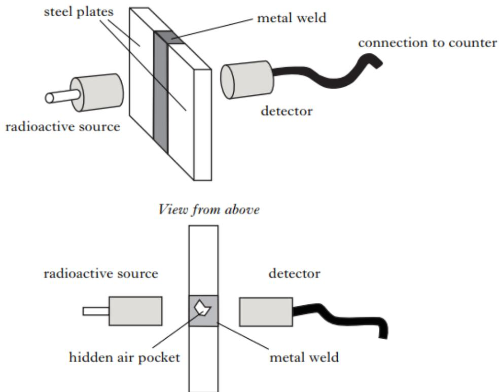
a) The radioactive source and detector are moved along the weld. How would the count rate change when the detector moves over an air pocket?
