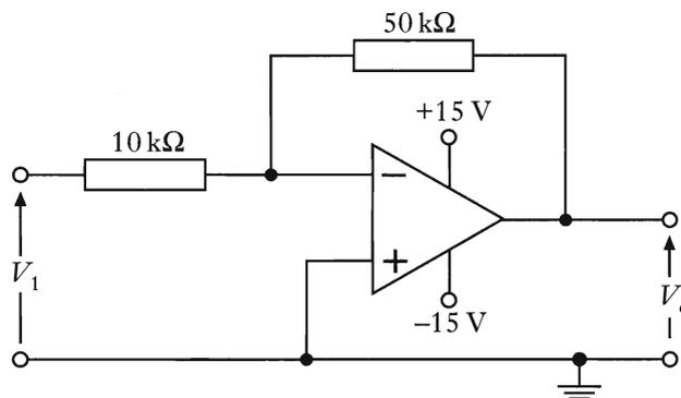
The input voltage  $V_1$  is +5 V. The most likely value for the output voltage  $V_0$  is
