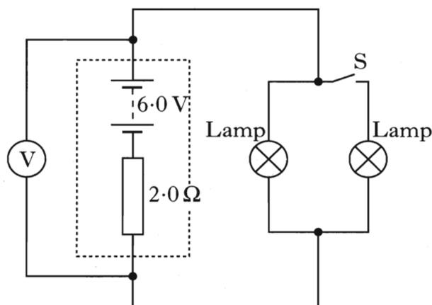
Describe and explain what happens to the reading on the voltmeter when switch S is closed.
