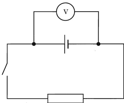
When the switch is open, the student notes that the reading on the voltmeter is 1.5 V. The switch is then closed and the reading falls to 1.3 V.
