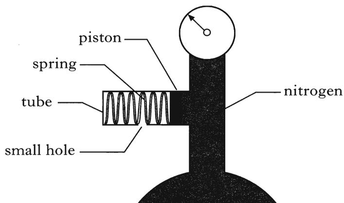
The piston of cross-sectional area  $4.0 \times 10^{-6} \text{ m}^2$  is attached to the spring. The piston is free to move along the tube.
