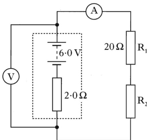
(i) Show by calculation that  $R_2$  has a resistance of 8.0 Ω.
