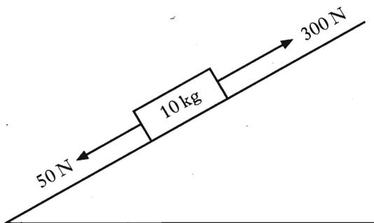
The box accelerates at  $10 \text{ m s}^{-2}$  up the plane.
