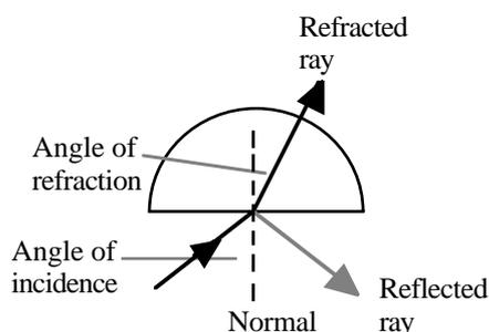
The light is said to be bent or **refracted** as it passes through the glass. This is due to the speed of light being less in glass than air. The ray will bend **towards** the normal.
