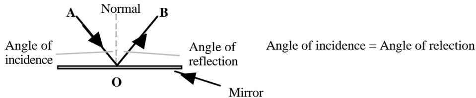
The **principle of reversibility of light** states that a ray of light which travels along any particular path from some point A to another point B travels by the same path when going from B to A, e.g. in the above diagram the ray travels from A to O to B. If the direction was reversed then the ray would follow B to O to A.
