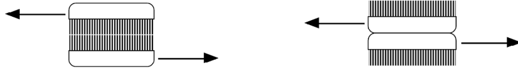
High Friction Sliding rough surfaces is like sliding the bristles of two brushes - it is difficult.
