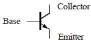
For a typical NPN transistor when the voltage across the base and emitter reaches 0.7 V it will switch on.
