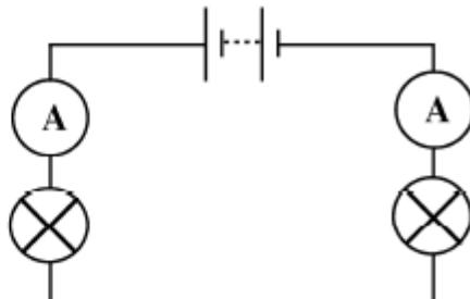
*To measure the current in each lamp, connect an ammeter in series with each lamp.*
