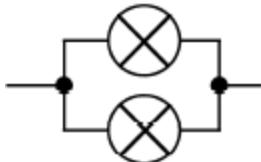
This diagram shows two lamps connected in parallel.
