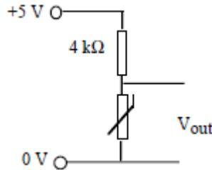
In the above circuit the reading at V<sub>out</sub> will increase as the temperature around the thermistor decreases. This increase in V<sub>out</sub> could allow another component or circuit to be activated. This is the principle behind frost detection circuits.
