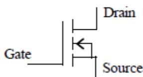
For a typical MOSFET when the voltage across the gate and source reaches 1.8V it will switch on
