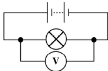
This circuit has a **voltmeter connected in parallel** across a lamp.
