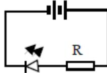
Note that the current in the above circuit will flow into the vertical line on the LED symbol. If the LED was reversed, current would not be able to flow and it would not light up.
