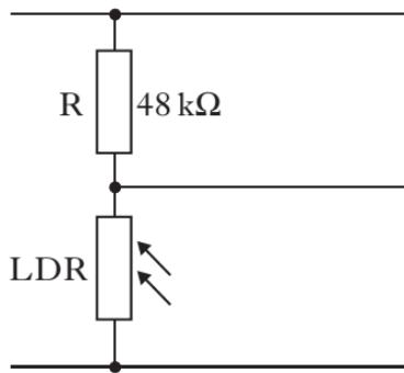
When the LDR has a resistance of  $2\text{k}\Omega$  the potential difference across it is 0.36V.
