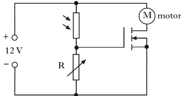
The resistance of the LDR on a cloudy day is  $3000\Omega$  and the variable resistor is set to a value of  $600\Omega$ .
