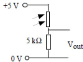
In the above circuit as the light level increases, the resistance of the LDR will decrease. This means that there will be less voltage needed across the LDR. As the available voltage has to be shared out between the LDR and the resistor, the voltage V<sub>out</sub> will increase. This increase in V<sub>out</sub> could allow another component or circuit to be activated. This is the principle behind automatic blinds.
