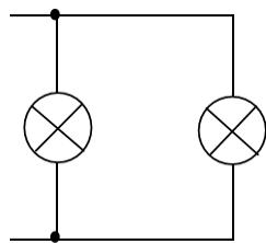
$$\begin{aligned}\frac{1}{R_T} &= \frac{1}{R_1} + \frac{1}{R_2} \\ &= \frac{1}{15.0} + \frac{1}{35.0} \\ R_T &= 10.5\ \Omega\end{aligned}$$
