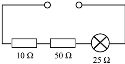
$$R_T = R_1 + R_2 + R_3$$
