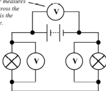
*To measure the voltage across each lamp, connect a voltmeter in parallel with each lamp.*
