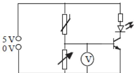
In the above circuit, when the temperature increases the resistance of the thermistor will decrease. This means there will be less voltage needed across the thermistor. As the available voltage has to be shared out between the thermistor and the variable resistor, the voltmeter reading will increase.
