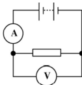
Use the **ammeter** to get a value of the **current** through the resistor.
