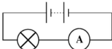
The circuit has an **ammeter inserted in series** with the lamp.
