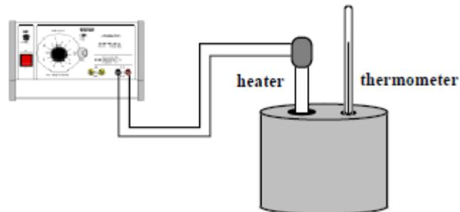
Specific heat capacity is calculated using the following equation:-
