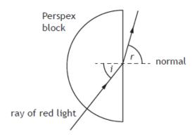
The angle of incidence i is then varied and the angle of refraction r is measured using a protractor.
