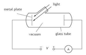
(a) When blue light is shone on the metal plate there is a current in the circuit. When blue light is replaced by red light there is no current.
