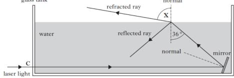
The refractive index of water for this laser light is 1.33.
